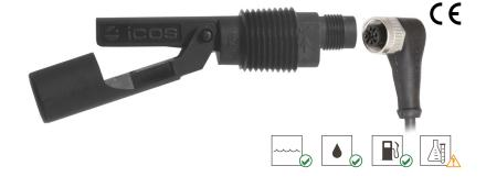
How it works Movement of the magnetic float opens/closes a hermetically sealed contact (reed switch).
