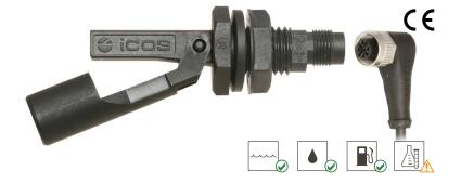
How it works Movement of the magnetic float opens/closes a hermetically sealed contact (reed switch).
