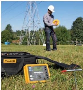
Faster setup, easier testing and deployment of wire reels and stakes.
