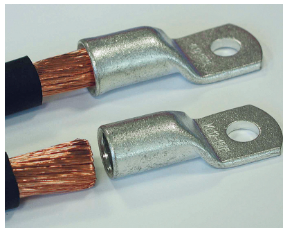
Picture 12: The funnel-shaped widening of the F cable lugs prevents a cross-sectional tapering of the cable caused by fraying
