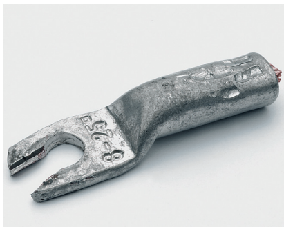
Picture 9: Indents made incorrectly due to unsuitable crimping tools, for example, can in the worst case cause a cable fire
