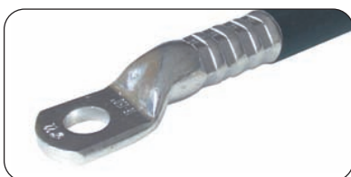
Picture 14: Tool code on the cable lug and imprinted code verify a correct crimp
