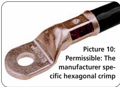
Picture 9: A cable lug resp. connector always needs to be crimped under consideration of the crimping direction and use of appropriate tools
