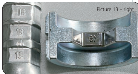
Picture 14: Tool code on the cable lug and imprinted code verify a correct crimp
