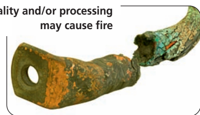
Picture 5: Incorrect or materials processed with inappropriate tools can cause heavy defects on installations resp. electrical equipment
