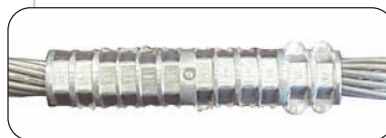
Picture 6: Cable lugs of poor quality and/or processing may cause fire
