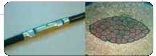
Picture 7: Gastight oval crimps provide for a permanent connection and good electrical conductivity. The ingress of fluid or a gaseous medium is not possible under normal atmospheric conditions. An oxidation of the individual crimped strands is prevented and an increase in resistance is avoided.
