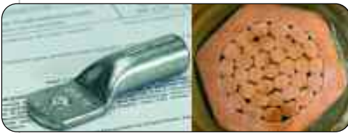
Picture 2: The standardized hexagonal crimp allows cable lugs and connectors per DIN 46235 to be crimped with certified crimping dies per DIN 48083 part 4.
