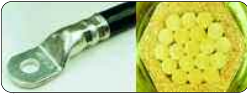
Picture 1: A hexagonal crimp is suitable for both copper and aluminium conductors. The advantage is the central force which is applied consistently from all directions.
