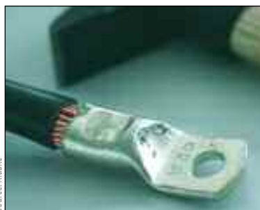
Incorrect cable lugs or the use of incorrect crimping tools can create serious safety defects in electrical installations and appliances
