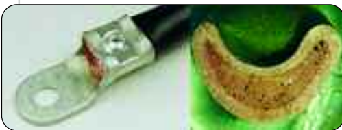
Picture 4: The intensive indent crimp is only guaranteed when matched materials are used despite the large outside diameters a permanent and „deep acting“ connection will be achieved.
