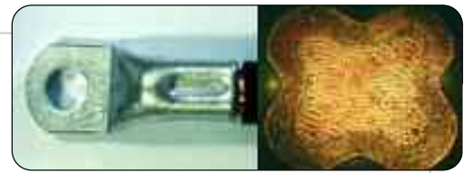
Picture 6: The quad point crimp is suitable for cable lugs and connectors with cross sections ranging from 10 mm 2 up to 300 mm 2 in combination with cable types per VDE 0295 classification 2, 5 and 6.
