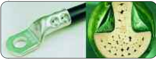
Picture 3: Indent (side indent) are always special application crimps which are primarily used for crimping fine stranded and compacted conductors to secure a permanent connection. The applied crimp profiles depend on the cross section of the conductor and type of cable lug.
